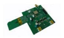
The AP6281 evaluation board showcases the capabilities of the SparkLAN SiP module, offering Wi-Fi and Bluetooth functions for separate testing. It supports an SDIO interface to connect to the host on the target platform, with options for SD Card Slot or Micro SD card slot, facilitating straightforward evaluation.
