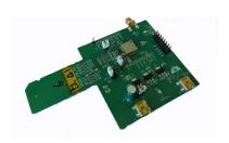
The AP6281 evaluation board is a universal development tool to highlight the capabilities of the AP6281 module.
