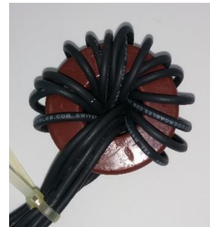
Figure 1: Core with winding under normal camera
