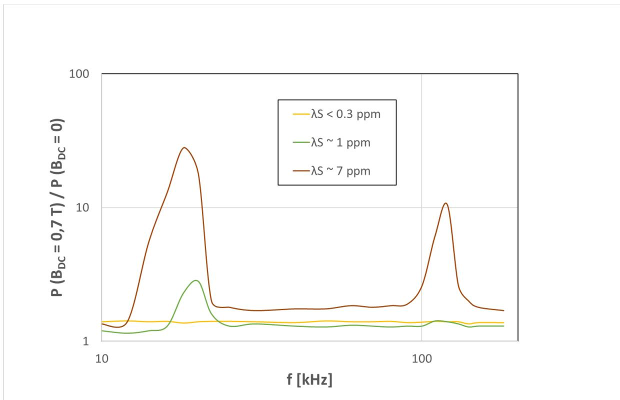
Fig.1: Toroidal cores with  $B_s \sim 1.2\text{T}$  and different magnetostriction: core losses  $P$  (at  $B_{AC} = 50\text{mT}$ ) as a function of exciting frequency, displayed as the ratio between with and without DC Bias.
