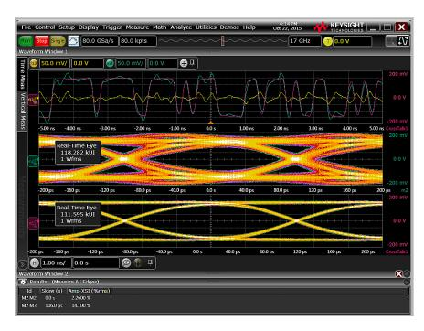
**Figure 5.** Before and after view of a victim waveform with FEXT using Advanced Signal Integrity software D9110ASIA.
