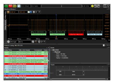
**Figure 3.** Protocol decoding of MIL-STD-1553 with D9110MILP showing a real-time trace, protocol decoding table, and packet details using a symbolic decode.
