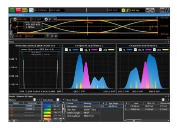
**Figure 4.** In addition to providing timing jitter separation, EZJIT Complete D9110JITA offers a comprehensive suite of vertical noise separation charts and phase noise measurements.
