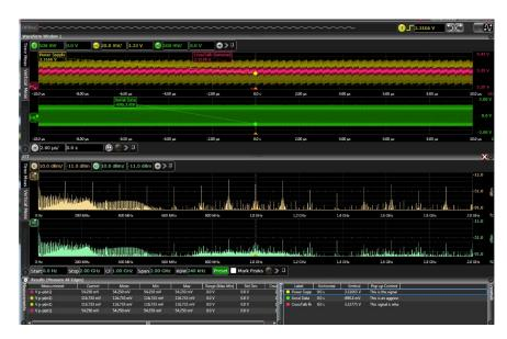
**Figure 6.** Output from the Power Integrity software application D9110POWA shows a reduction in the noise on a 3.3 V supply after the effects of removing the switching loads.
