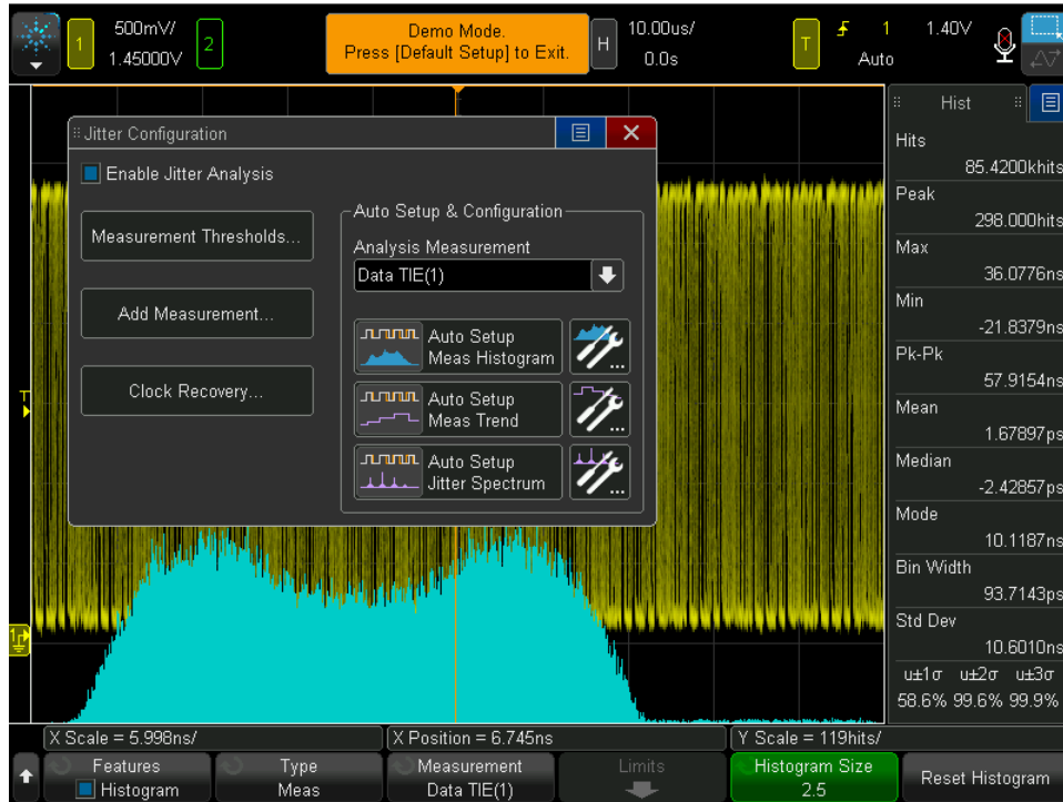
Figure 5. Jitter histogram using DSOX6004JIT High-Speed / Jitter Better Bundle.
