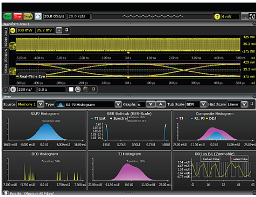
Figure 9. Real-world jitter measurements with the Infiniium S-Series oscilloscopes.
