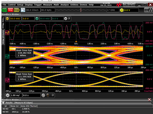
Figure 10. Before and after view of a victim waveform with FEXT. The top plot shows the victim waveform in green, the aggressor in orange, and the crosstalk removed waveform in red. The middle plot is the eye diagram of the victim with the bulging indicative of FEXT. The bottom plot is the eye diagram of the victim after removing crosstalk.
