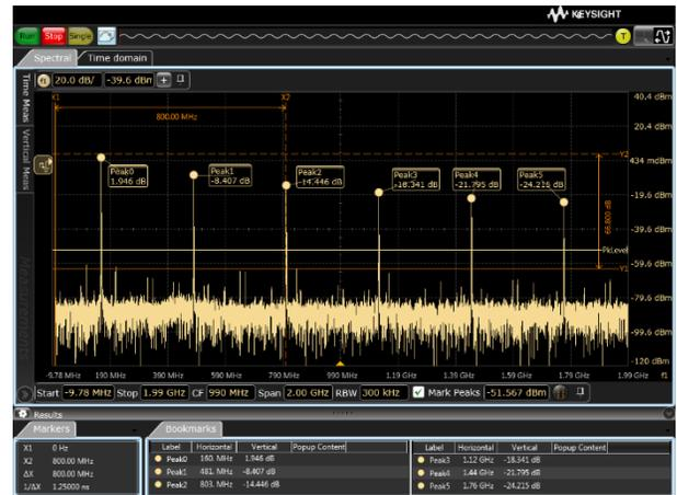
Peak readouts in the FFT plot.
