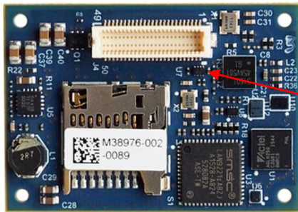
Driver chip installed on board
