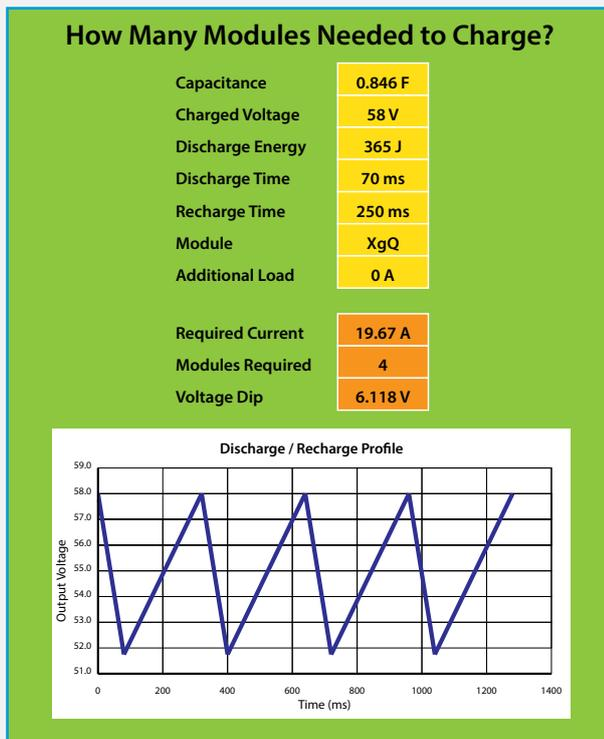
So four XgQ modules will meet the desired charge and discharge profiles for this application. These will fit in a UX6 UltiMod chassis, giving a unique part number of UX6QQQ00.
