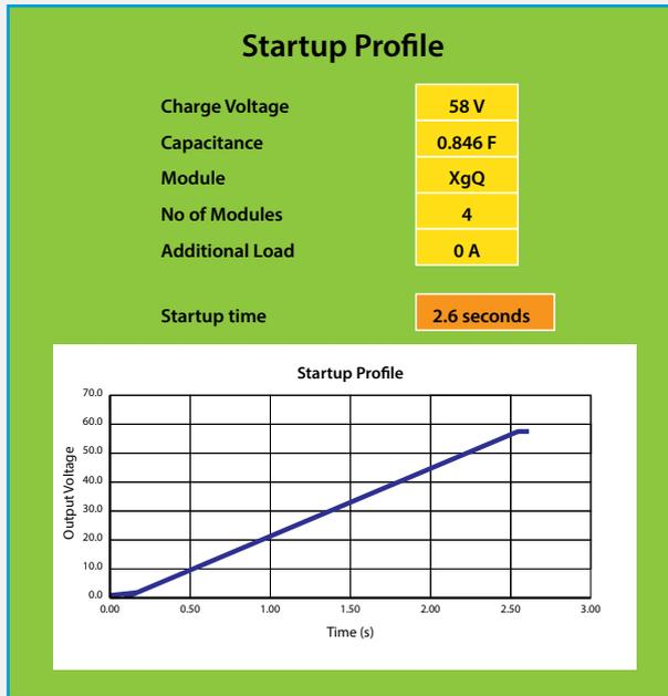
The capacitance is charged in 2.6 seconds, within specification.
