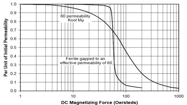
Fig. 1. Saturation curve of a gapped ferrite and a powder core with the same effective permeability [6].
