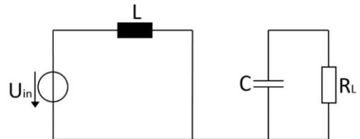
Fig. 8. Boost converter circuit in the state of high gate (PWM) signal.
