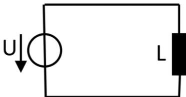
Fig. 3. Test circuit for a transient simulation of saturation.
