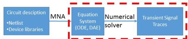
Fig. 2. Transient circuit simulation within a SPICE software.
