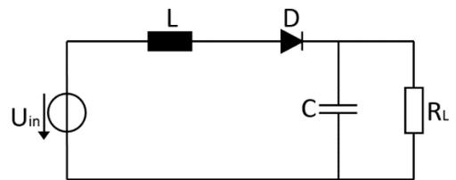
Fig. 9. Boost converter circuit in the state of low gate (PWM) signal.
