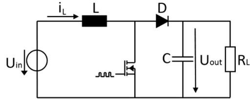
Fig. 7. Boost converter circuit.
