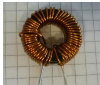
Fig. 5. Inductor: Core 77310-A7 (KoolM $\mu$  material),  $N=57$  turns.
