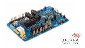
A small form factor evaluation board, powered by USB, that exposes all the BX3100 and BX3105 modules' pin interfaces via headers. It has a UART-to-USB converter at 1Mb/s for direct connection of the UART to a PC.
