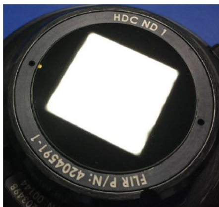
Figure 6-9: HDC lens with ND1 filter screwed into the back
