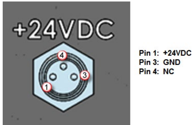
Figure 5-1: A6705 Power Input Pinouts
