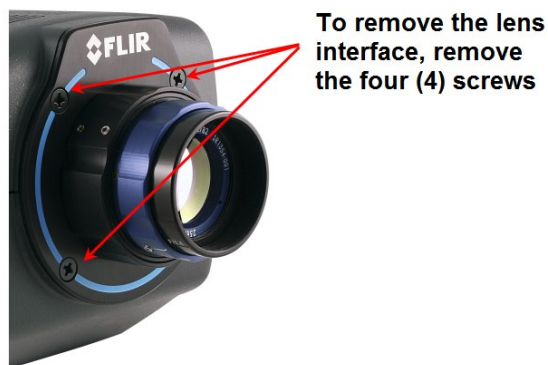
Figure 6-8: Removable lens mount
