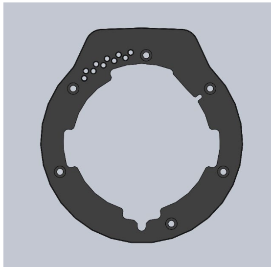
Figure 6-12. FLIR 5-Tab FPO Motorized Focus Lens Bayonet
