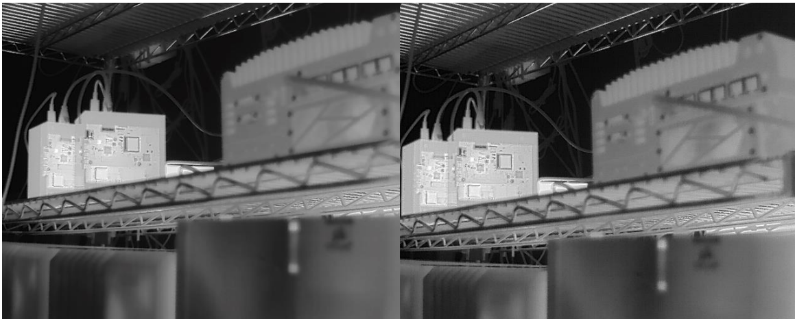
FIGURE 31: EXAMPLE IMAGES SHOWING VALUES OF DDE+ SUPPRESSION (0.1 LEFT AND 1.2 RIGHT)
