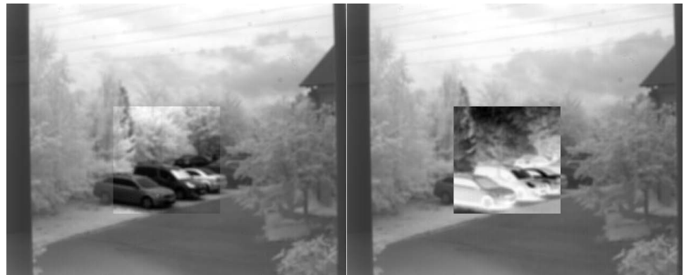
Figure 98: Left: Auto contrast applied to a ROI in the usual way, right: auto contrast with the ContrastAutoIntensity values reversed.
