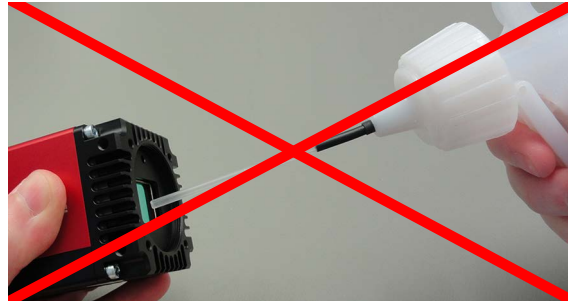
Figure 111: How not to use compressed air
