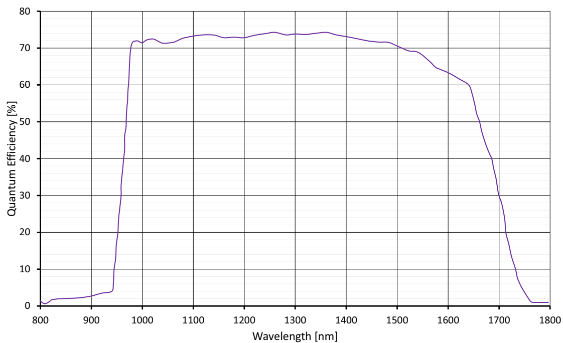
Figure 22: Goldeye CL-032 SWIR TEC1 absolute QE
