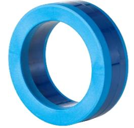
Magnetec developed special cores with own developed CoolBLUE annealing with the special purpose to absorb the high frequency noise – we call our CoolBLUE cores inductive absorber as the noise is transferred to thermal energy instead of unwanted discharges at the motor bearings.
