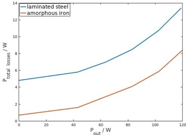
**Fig. 7:** Transformers losses versus output power ( $U_{in} = 230V$ )
