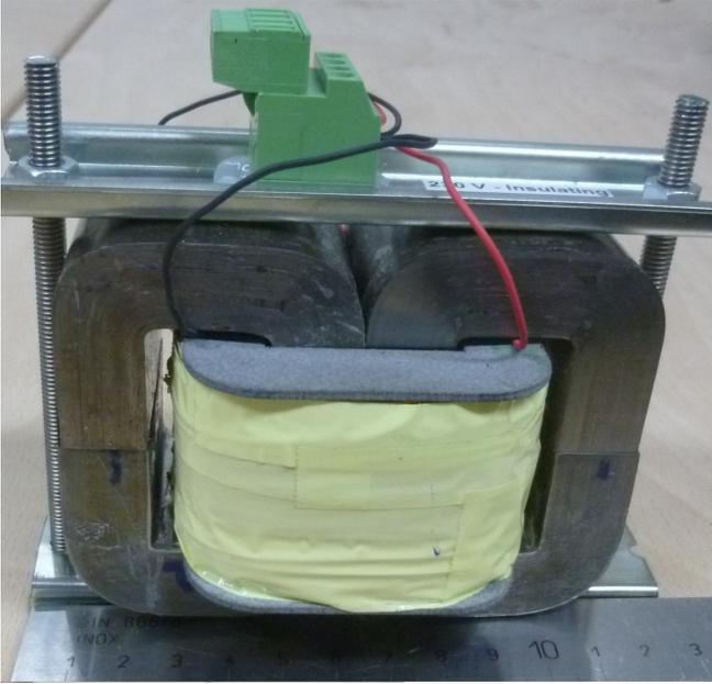
**Fig. 5:** Amorphous transformer 230V, 50Hz, 110VA, 1:1
