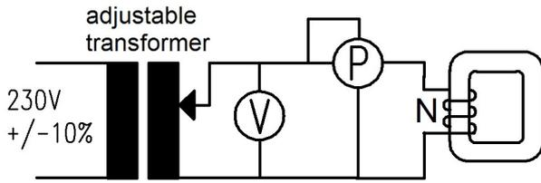
**Fig. 3:** Cut core power loss setup
