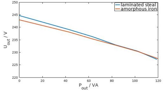
**Fig. 6:** Transformers output voltage over load ( $U_{in} = 230V$ )
