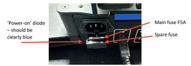
Remove the fuse from the rear pocket and insert the spare fuse from the front pocket. Remember to buy a new spare fuse – a fast-blow 5 A fuse.
