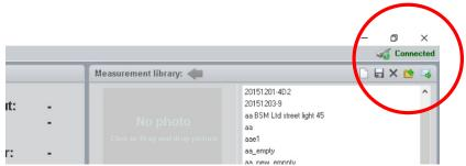
You can connect and disconnect the USB without restarting the "Viso Light Inspector" software, as the connection is always established automatically as soon as the USB connector is plugged in and vice versa.
