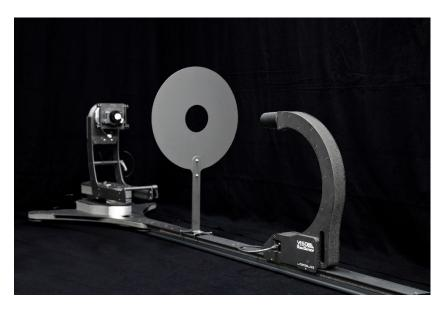
You may also consider the standard Viso accessory LabDisc to prevent straylight in your lab. This unit sits permanently on the tripod/LabRail stem and limits the sensor field-of-view to a minimum.
