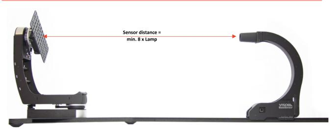
For example, for a lamp with a 20 cm diagonal illuminating surface (the photometrical center being in the middle of the diffuse disc), the distance from center of rotation of the gonio to the sensor should be at least 160cm (20cm x 8). See more in "Guidelines - building a lighting laboratory".
