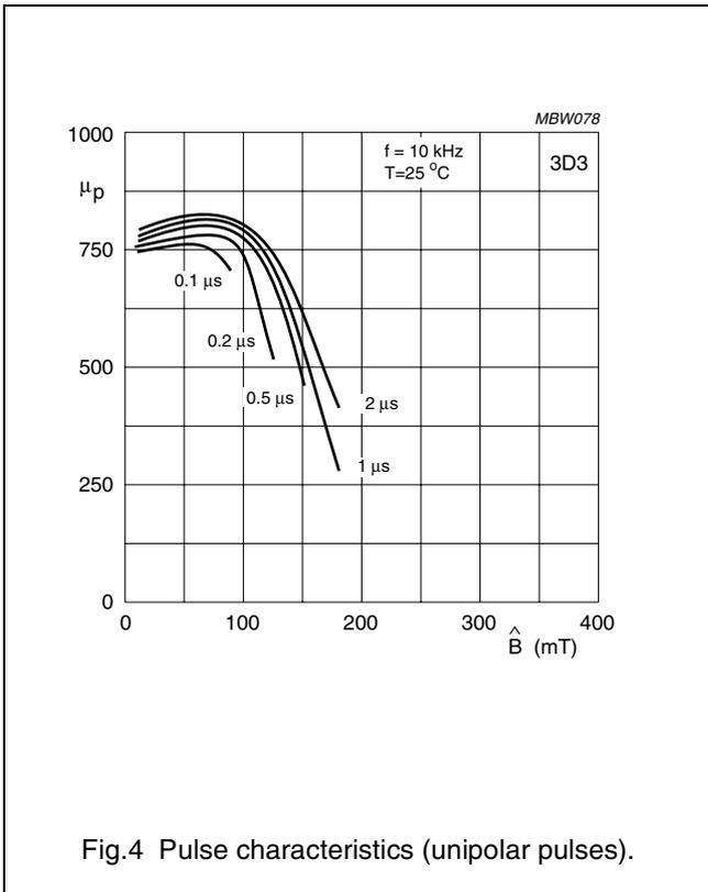
Fig.4 Pulse characteristics (unipolar pulses).
