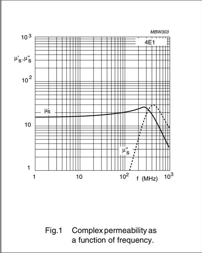
Fig.1 Complex permeability as a function of frequency.
