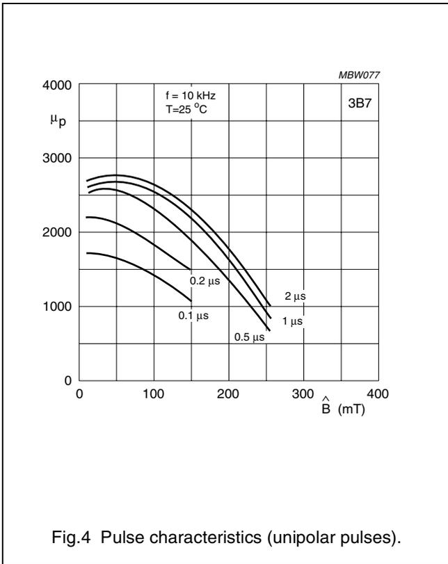
Fig.4 Pulse characteristics (unipolar pulses).
