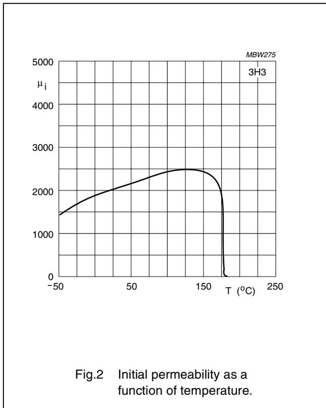
Fig.2 Initial permeability as a function of temperature.
