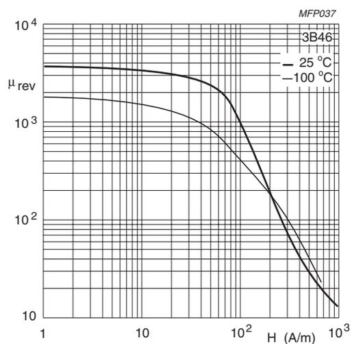
Fig.4 Reversible permeability as a function of magnetic field strength.
