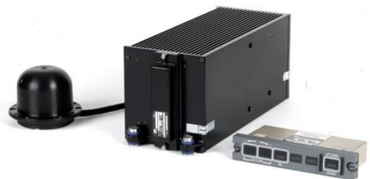
Fig. 3: APIRS™, Tactical grade AHRS by Safran Electronic & Defense
