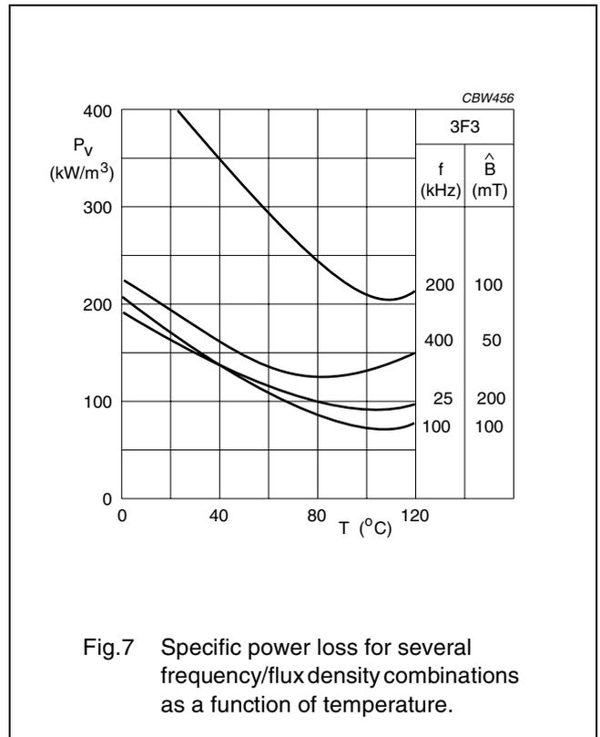
Fig.7 Specific power loss for several frequency/flux density combinations as a function of temperature.
