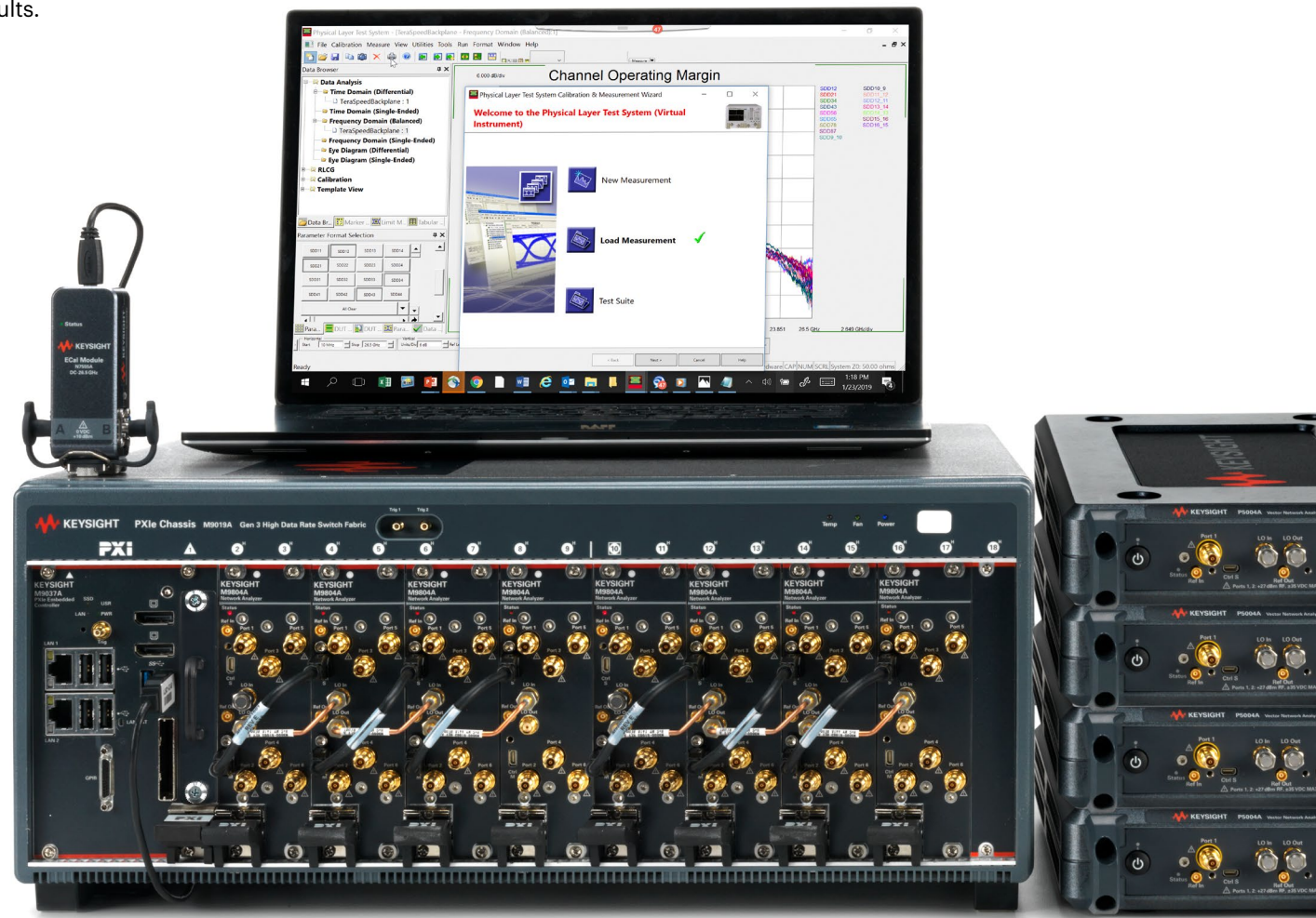
M9019A PXI Chassis with M9804A PXI Vector Network Analyzers
