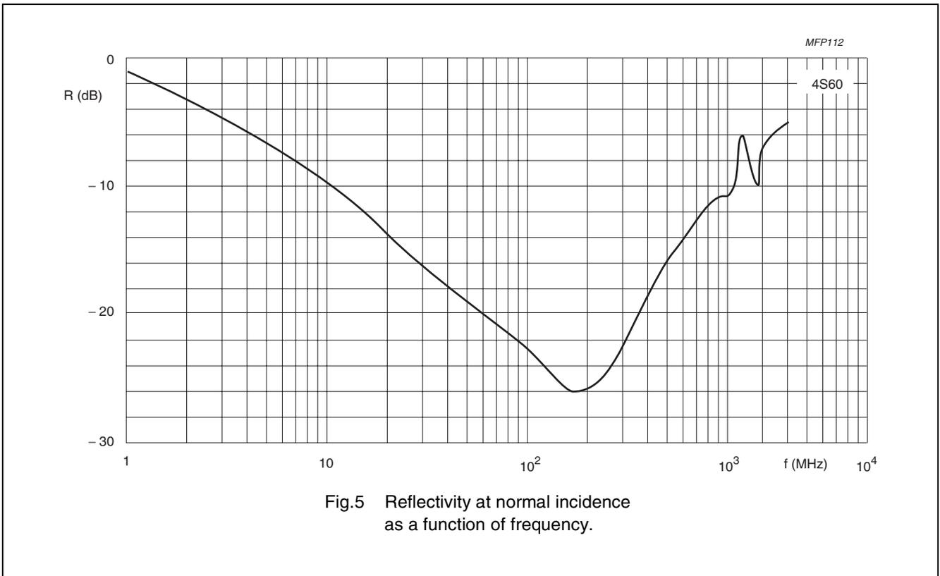
Fig.5 Reflectivity at normal incidence as a function of frequency.
