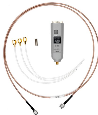
N7020A power rail probe
