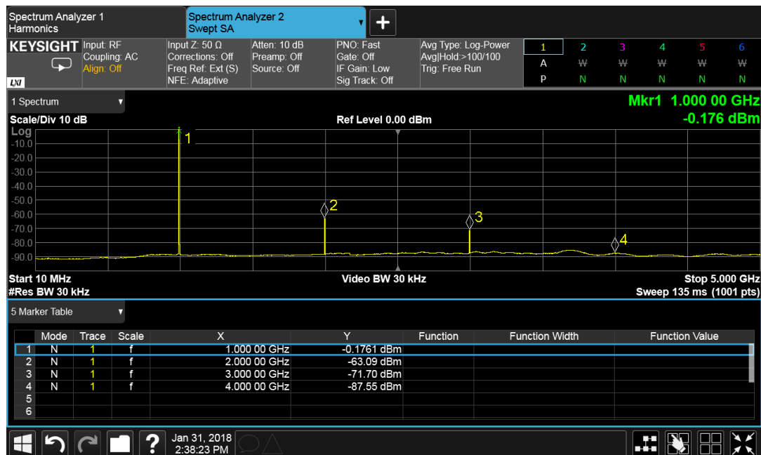
Figure 1-4. Spectrum analysis with frequency and amplitude readouts
