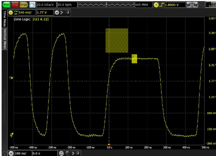
**Figure 1.** InfiniiScan D9110SCNA measurement finder triggers on all edges, then only displays signals with rise times less than 50 or greater than 70 ns.
