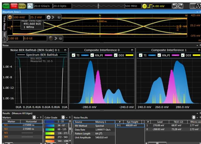
**Figure 4.** In addition to providing timing jitter separation, EZJIT Complete D9110JITA offers a comprehensive suite of vertical noise separation charts and phase noise measurements.
