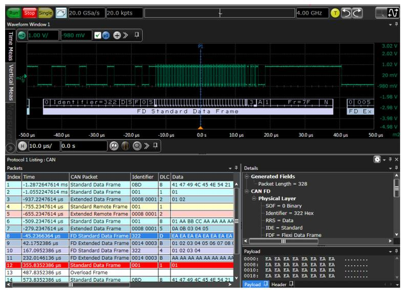
Figure 2. Controller Area Network (CAN) bus decode using Infinium D9110AUTP software.
