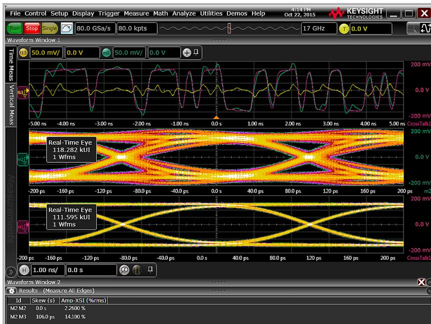
Figure 5. Before and after view of a victim waveform with FEXT using Advanced Signal Integrity software D9110ASIA.
