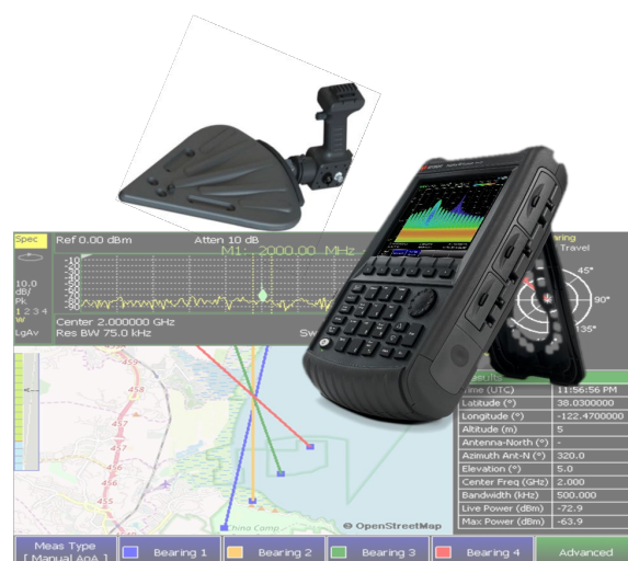
Moving a FieldFox connecting with the directional antenna, one can trace the cross-section of trajectory lines (or “bearings”) of the interference. Overlaying this data onto the GPS map allows for precise pinpointing of the interference
