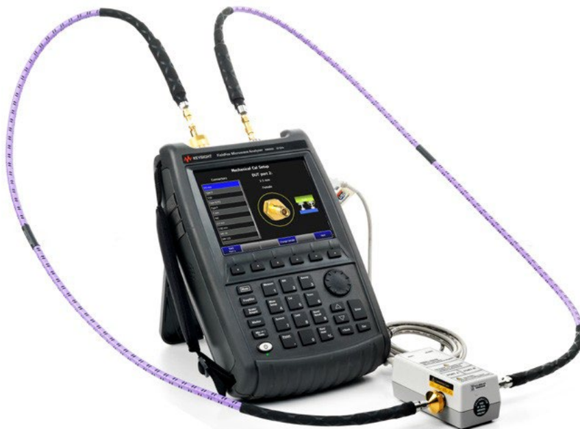
Perform fast and accurate calibrations using ECal
