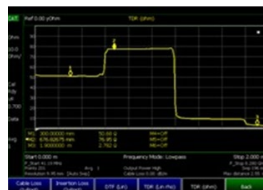
Gain insight into faults with TDR measurement
