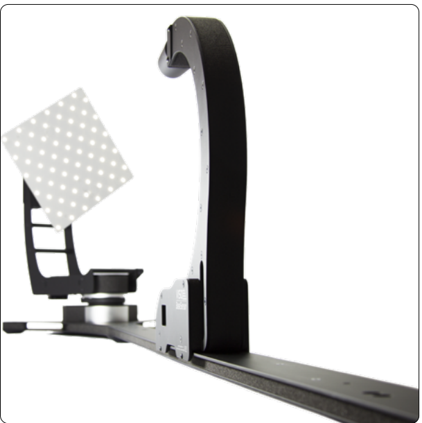
BaseSpion For medium-sized light sources up to 9 kg (20 lbs). Spectrometer sensor slides on a tabletop rail.
