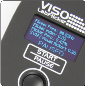
OLED display gives live flicker results during measurement
