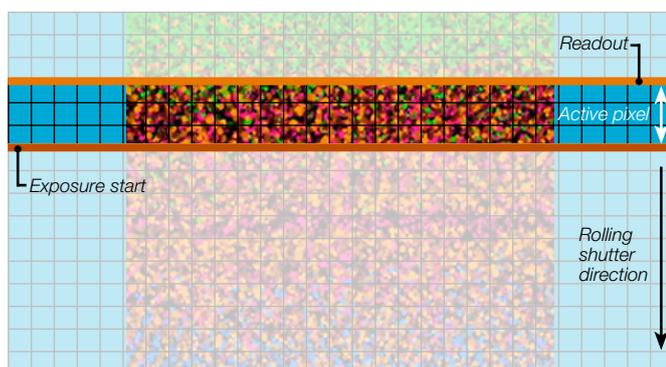
**Figure 1:** Rolling Shutter mode. The highlighted window of pixel rows is exposed to light. This band sweeps from the top to the bottom of the sensor and can be synchronized to the sweep of an illumination laser.
