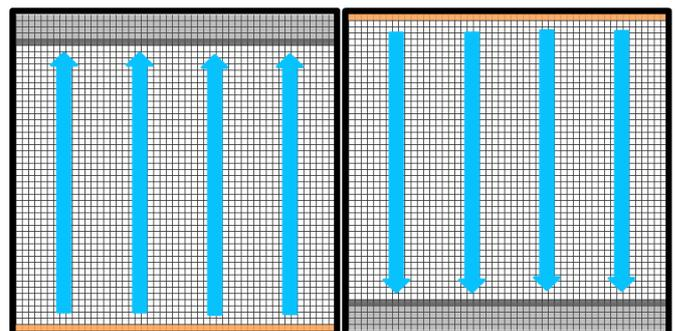
**Figure 2:** LightScan PLUS enables the rolling shutter to scan the sensor from top to bottom or vice versa in one continuous sweep. This is also known as Single Port Readout.
