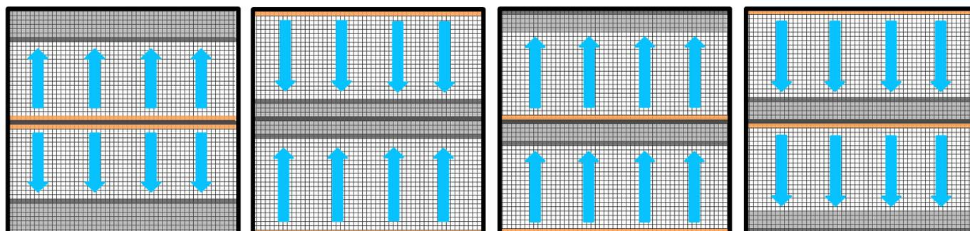
**Figure 3:** Multiple 'dual laser' scanning options available. The standard rolling shutter scan mode (Centre outwards in both directions simultaneously) is illustrated on the left along with the three additional scanning options.
