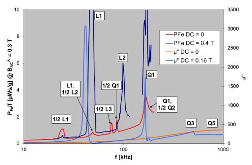
Fig.2: Toroidal core with  $B_s \sim 1.2T$  and  $\lambda_s \sim 7$ ppm: core losses  $P_{Fe}$  and imaginary part of permeability  $\mu$ " as a function of exciting frequency, both with and without DC Bias. L indicates longitudinal, Q transversal resonance modes; the number the order.
