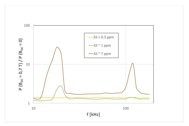
Fig.1: Toroidal cores with  $B_S \sim 1.2T$  and different magnetostriction: core losses P (at  $B_{AC} = 50mT$ ) as a function of exciting frequency, displayed as the ratio between with and without DC Bias.
