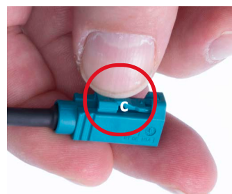
Figure 22: Pressing down the latch (c) of the FAKRA coaxial connector
